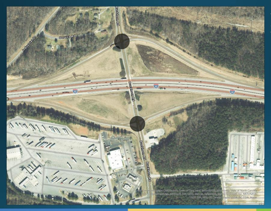
The NCDOT will design and install a traffic signal at each ramp of the interchange of I-40 and SR 1114 (Buckhorn Road) in Mebane.
